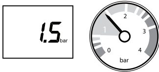
Fig.51 Restore water pressure
